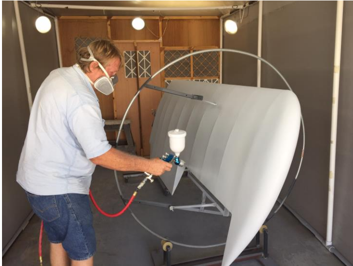
Above – Audie applies base coat to one of the four wings. Right – Audie’s trusty helper, Lon Beasley, helps to keep paint mixed-up and ready.
