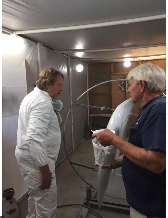
Above – Audie applies base coat to one of the four wings. Right – Audie’s trusty helper, Lon Beasley, helps to keep paint mixed-up and ready.
